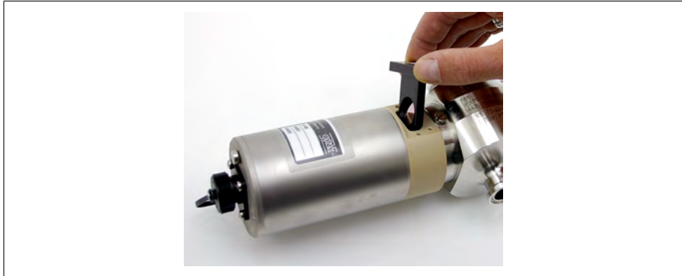
Fig. 18: Inserting the calibration filter's filter holder
