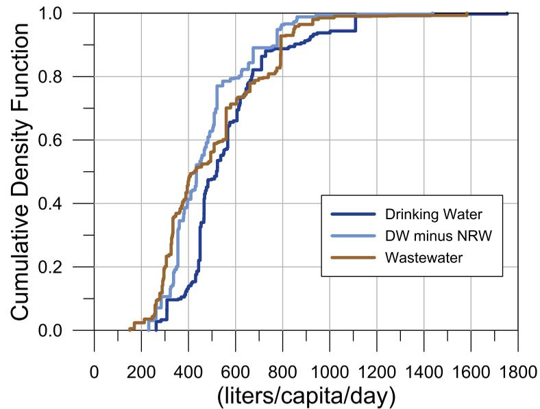
**Figure 2.** The dark blue and brown lines show the distribution of weighted, per capita drinking water, and wastewater averages, respectively. The cumulative distribution function is based on the total service populations of utility data received. The light blue line shows the CDF for drinking water flux after removing non-revenue water (NRW).
