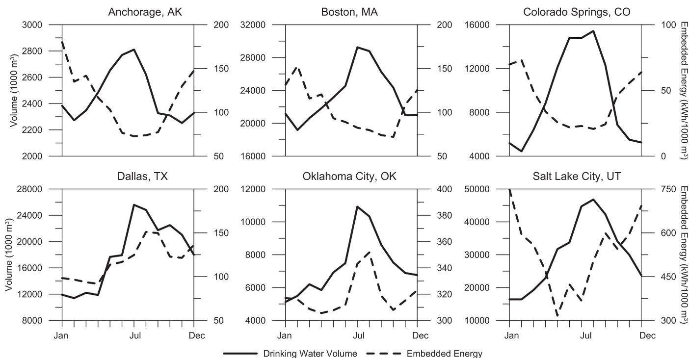
**Figure 11.** Cities in colder climates that use natural gas as part of their treatment and distribution processes for drinking water have much higher embedded energy in the winter than in the summer. The shapes of these curves show the importance of natural gas in the embedded energy of some cities' drinking water.
