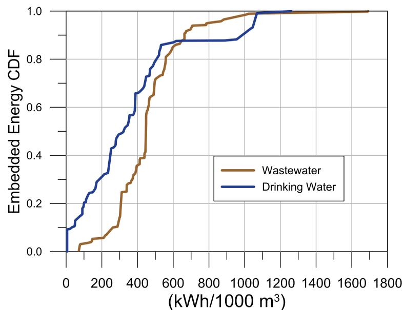
**Figure 3.** Cumulative distribution functions for the embedded energy of drinking water and wastewater resources show a skewed right tail of the distribution where larger embedded energy is required.
