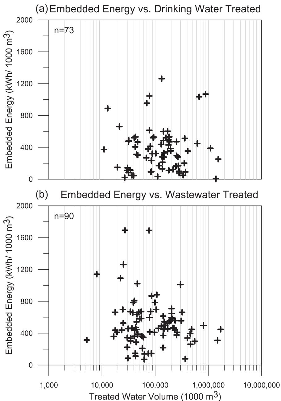
**Figure 4.** The embedded energy demand associated with total treated volume for both drinking water and wastewater does not suggest any economies of scale with regards to energy per treated volume.
